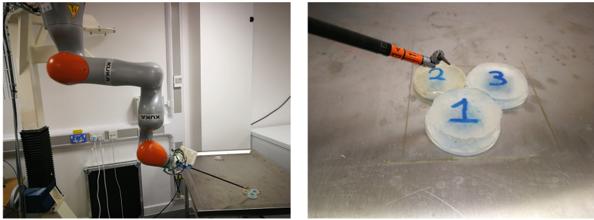
(a) Actual configuration of slave while in contact with active constraints. (b) Focus on the area of the active constraints.
